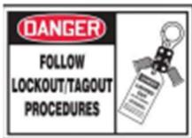
Before servicing dumper, be sure that all sources of energy have been shut off, all potential hazards have been eliminated, and the dumper is locked-out and tagged-out in accordance with OSHA and ANSI requirements
