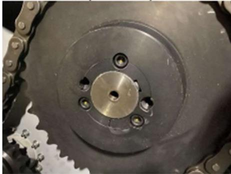
8. Ensure the motor/gearbox/gearbox mounting plate bolts are tight.
