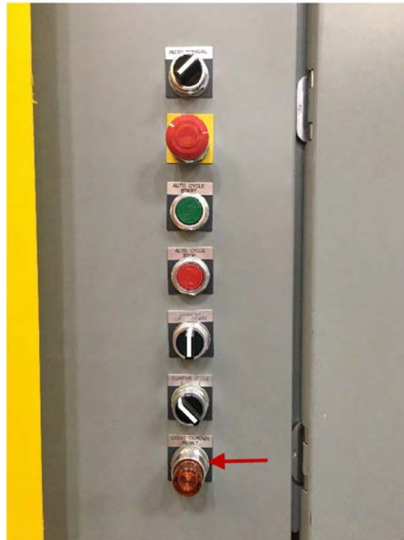
Figure 2: If the Light Curtain Reset amber push button is illuminated, depress the push button to reset the light curtains.
