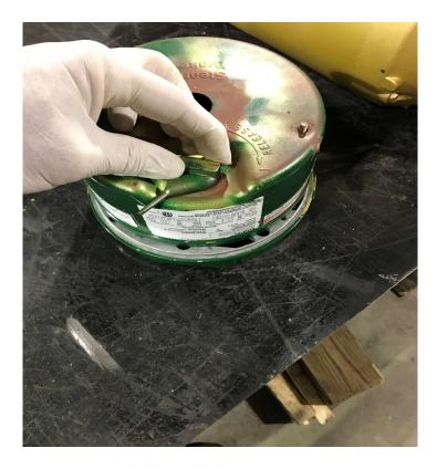
Remove the two small nuts. Hold the brake release to the position in picture And pull off cover.
