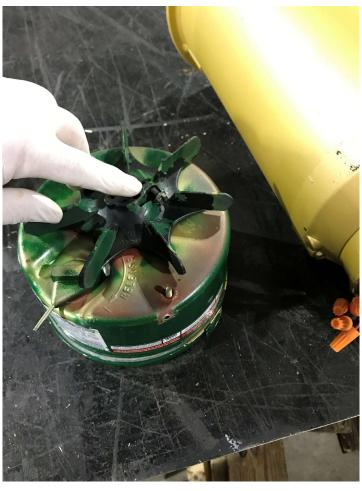
Loosen the screw and pry the fan off.
