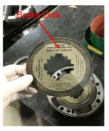
Remove the pressure plate, Disk, Pressure plate, Disk, Pressure plate, Disk and then the wavy plate.
