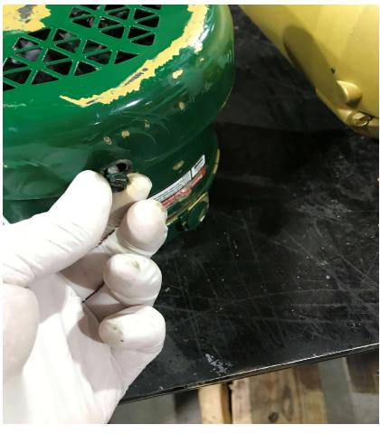
Remove the three screws and pull fan cover off
